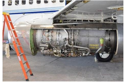
The Safety net that I thought about later was to simply spread a rag out under the component you are installing in order to catch anything that might be dropped. Just a minute of time to think what could go wrong would have saved me a lot of stress that night. I call that time, “**a minute for Safety.**”
